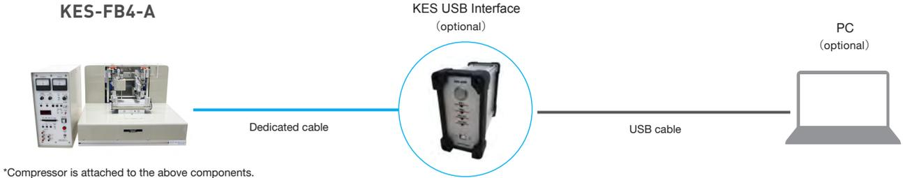
\*Compressor is attached to the above components.
